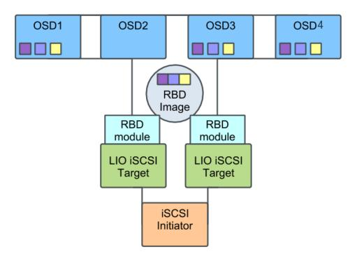
FIGURE 9.2: CEPH CLUSTER WITH MULTIPLE ISCSI GATEWAYS
