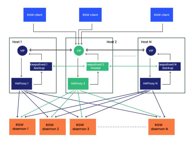
FIGURE 8.1: HIGH AVAILABILITY SETUP FOR OBJECT GATEWAY
