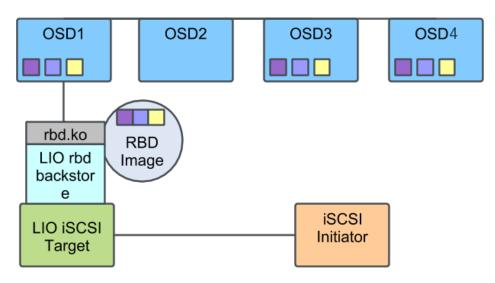
FIGURE 9.1: CEPH CLUSTER WITH A SINGLE ISCSI GATEWAY
