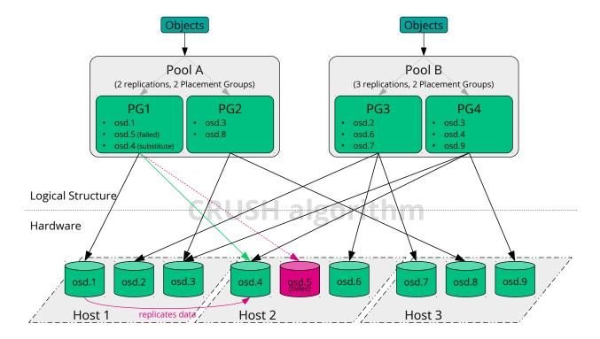
FIGURE 1.2: SMALL SCALE CEPH EXAMPLE
