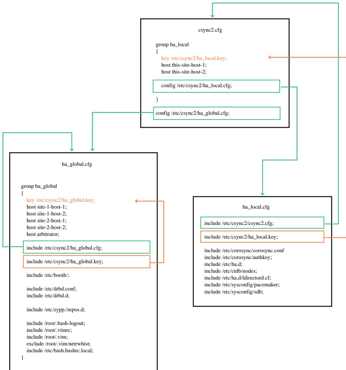
FIGURE 5.1: EXAMPLE CSYNC2 SETUP FOR GEO CLUSTERS
