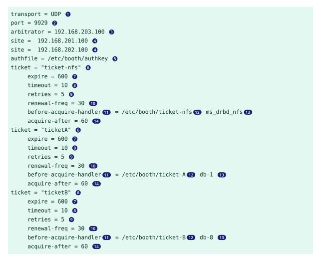
The transport protocol used for communication between the sites. Only UDP is supported, but other transport layers will follow in the future. Currently, this parameter can therefore be omitted.
