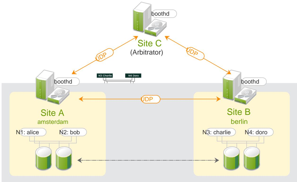
FIGURE 2.1: TWO-SITE CLUSTER (2X2 NODES + ARBITRATOR)
