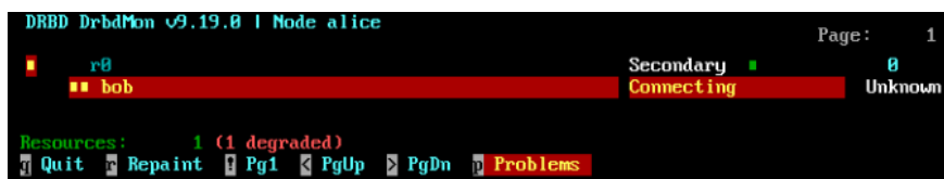
FIGURE 23.5: SHOWING A BAD CONNECTION BY drbdmon
