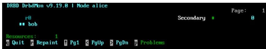
FIGURE 23.4: SHOWING A GOOD CONNECTION BY drbdmon
