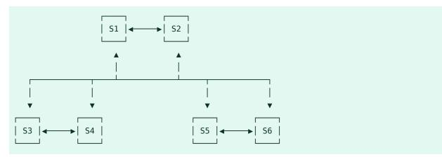
In *Example 5.6, "Six replicas"*, each pair is in a separate location. S1 and S2 are the suppliers, and S3, S4, S5, and S6 are consumers of S1 and S2. Each pair of servers replicate to each other. S3, S4, S5 and S6 can accept writes, though most of the replication is done through S1 and S2. This setup provides geographic separation for high availability and scaling.
