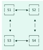
*Example 5.5, "Four supplier replicas"* has four supplier replicas, which all synchronize to each other. These could be in four datacenters, or two servers per datacenter. In the case of one node per data center, each node should be able to support 100% of client load. When there are two per datacenter, each one only needs to scale to 50% of the client load.
