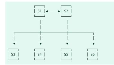
In *Example 5.7, "Six replicas with read-only consumers"*, S1 and S2 are the suppliers, and the other four servers are read-only consumers. All changes occur on S1 and S2, and are propagated to the four replicas. Read-only consumers can be configured to store only a subset of the database, or partial entries, to limit data exposure. You could have a fractional read-only server in a DMZ, for example, so that if data is exposed, changes can not propagate back to the other replicas.
