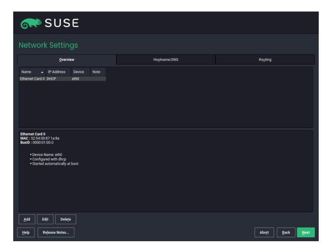
A system analysis is performed, where the installer probes for storage devices, and tries to find other installed systems. If the network was automatically configured via DHCP during the start of the installation, you will be taken to the registration step.
