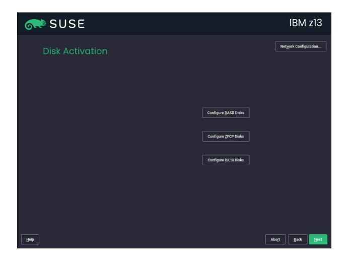
Configure the attached hard disks. Select DASD, Fibre Channel Attached SCSI Disks (zFCP), or iSCSI for the installation of SUSE Linux Enterprise Server. The DASD and zFCP configuration buttons are only available if the corresponding devices are attached. Proceed with *Next* to set up the selected disk type. For more information, refer to *Book "Deployment Guide"*, *Chapter 8 "Installation steps"*, *Section 8.5 "IBM Z: disk activation"*.
