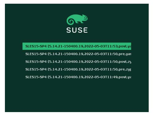
FIGURE 10.1: BOOT LOADER: SNAPSHOTS
