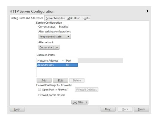
FIGURE 42.3: HTTP SERVER CONFIGURATION: LISTEN PORTS AND ADDRESSES
