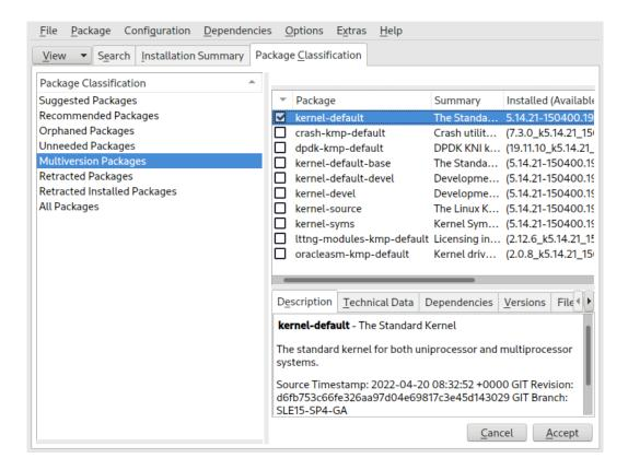
FIGURE 27.1: THE YAST SOFTWARE MANAGER: MULTIVERSION VIEW
