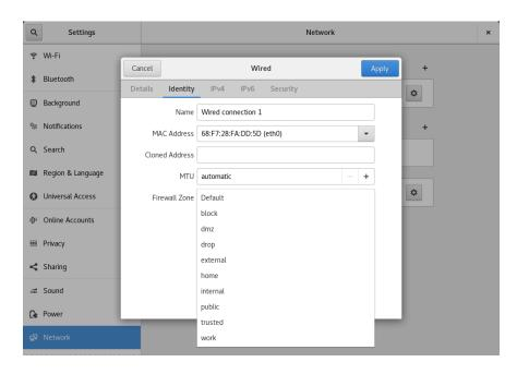
FIGURE 31.2: firewalld ZONES IN NETWORKMANAGER
