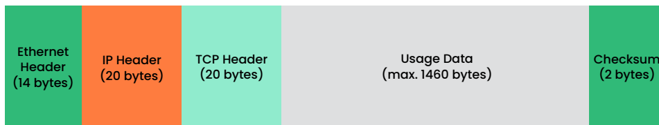
FIGURE 23.2: TCP/IP ETHERNET PACKET
