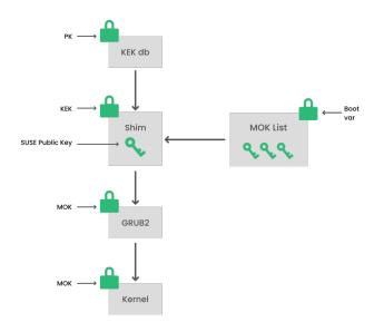
FIGURE 17.2: UEFI: SECURE BOOT PROCESS
