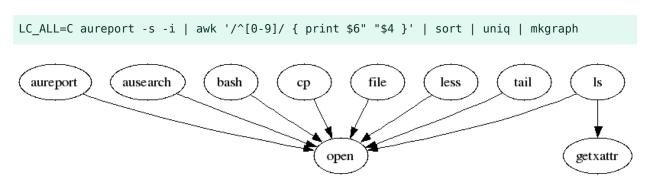
FIGURE 44.2: FLOW GRAPH—PROGRAM VERSUS SYSTEM CALL RELATIONSHIP
