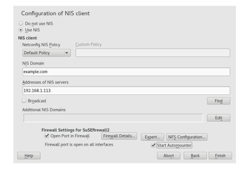
FIGURE 3.6: SETTING DOMAIN AND ADDRESS OF A NIS SERVER
