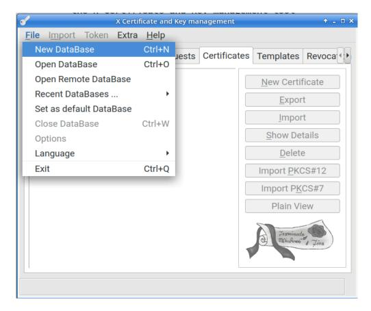
FIGURE 25.1: CREATE A NEW XCA DATABASE
