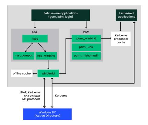
FIGURE 7.1: SCHEMA OF WINBIND-BASED ACTIVE DIRECTORY AUTHENTICATION
