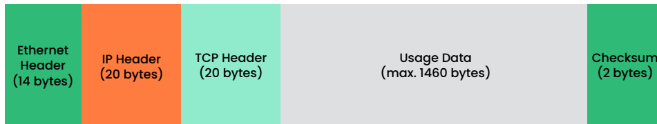
FIGURE 23.2: TCP/IP ETHERNET PACKET
