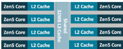
FIGURE 3: CCX WITH EIGHT ZEN5 COMPUTE CORES AND 32 MB SHARED L3 CACHE
