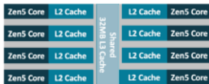
Figure 2-3: CCX with eight Zen5 compute cores and 32 MB shared L3 cache (corresponds to Figure 2-1, above)
