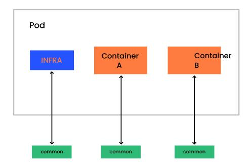
Each container in a pod has its own instance of a monitoring program. The monitoring program watches the container's process and if the container dies, the monitoring program saves its exit code. The program also holds open the tty interface for the particular container. The monitoring program enables you to run containers in the detached mode when Podman exits, because this program continues to run and enables you to attach tty later.
