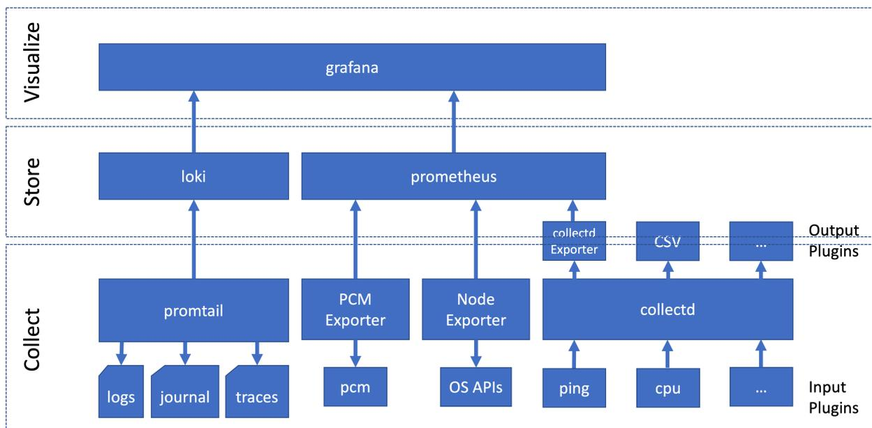
FIGURE 1: MONITORING COMPONENTS
