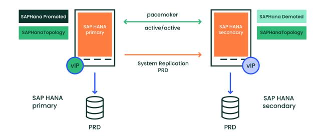
Performance optimized, including read-enabled on the secondary site (A => B)
