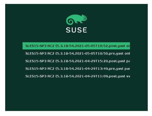
FIGURE 7.1: BOOT LOADER: SNAPSHOTS
