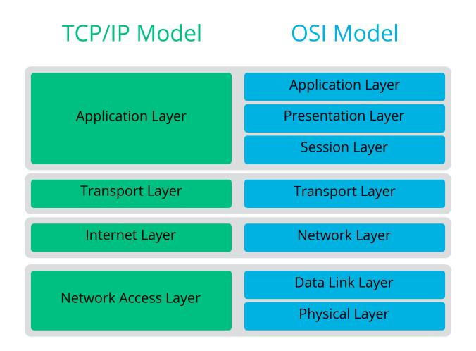
FIGURE 19.1: SIMPLIFIED LAYER MODEL FOR TCP/IP
