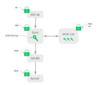
FIGURE 13.2: UEFI: SECURE BOOT PROCESS
