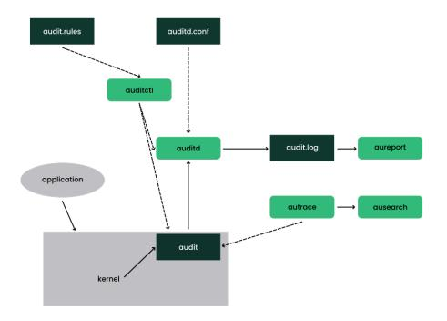
FIGURE 44.1: INTRODUCING THE COMPONENTS OF LINUX AUDIT
